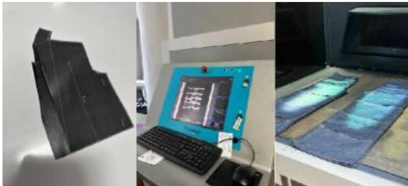
Figure 10. Production processes: small-scale pattern, Control Panel-Laser System, Laser Distress.
