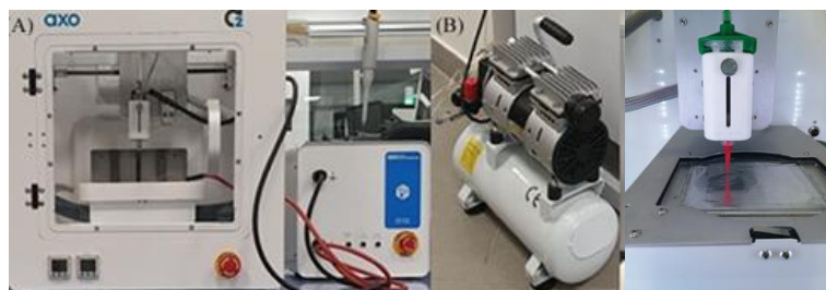
Figure 1: Extrusion Based Bioprinting setup for the Axo Biosystem Printer
