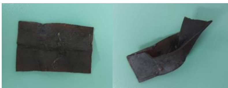
Figure 1. Sample of fermented bioleather after 10,000 cycles.
