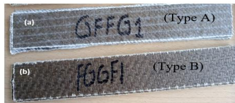
Figure. 1. Hybrid composite: a) Flax fiber fabrics positioned in the core layers, b) Flax fiber fabrics were positioned in the outer layers
