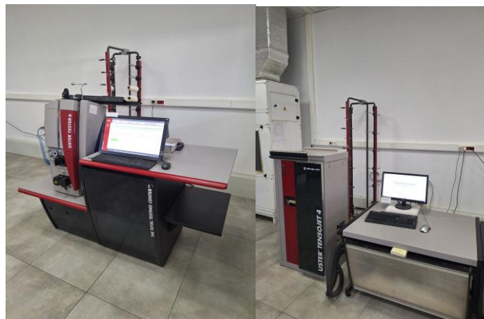
Figure 2. Testing equipment used for yarn characterization
