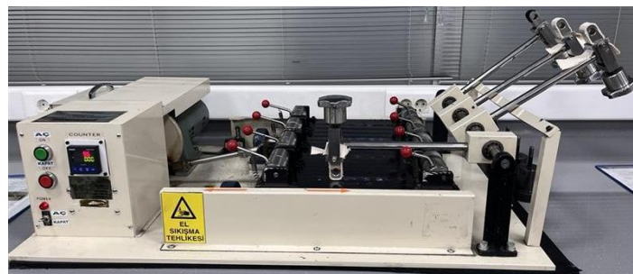
Figure 1. Surface Abrasion Test Device
