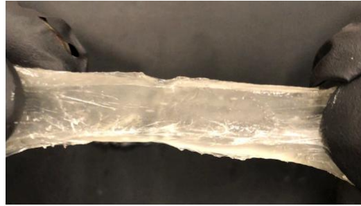
Figure 4. Tensile test images of the healed hydrogel sample
