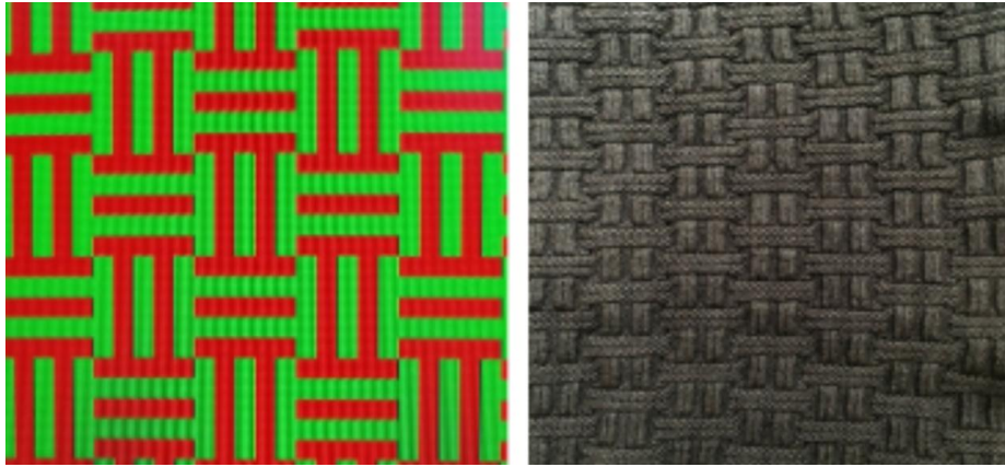
Figure 2. APEX Digital Knitting Pattern and Structural Representation of Sample B
