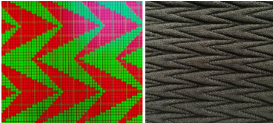
Figure 3. APEX Digital Knitting Pattern and Structural Representation of Sample C
