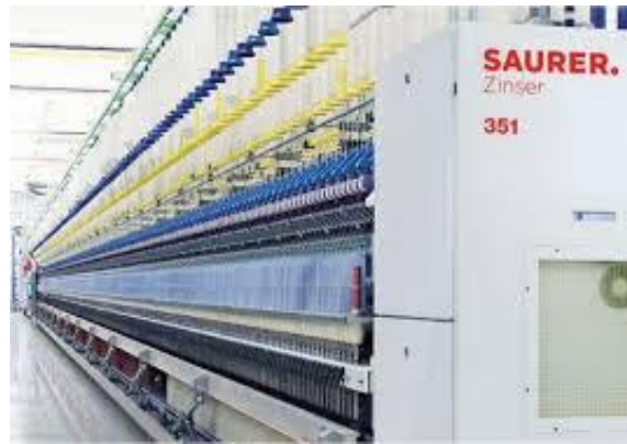
Figure 1. Ring spinning machine used for yarn production
