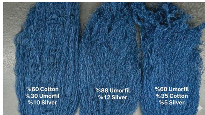
Figure 10. Photographs of yarn samples dyed with reactive dye
