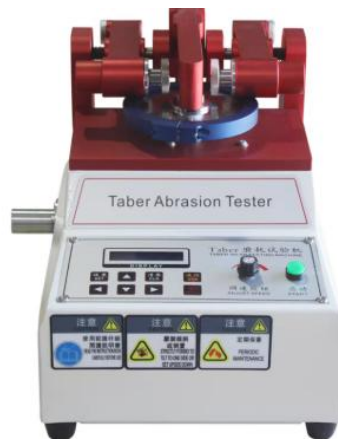
Figure 2. Taber Abrasion Test Device
